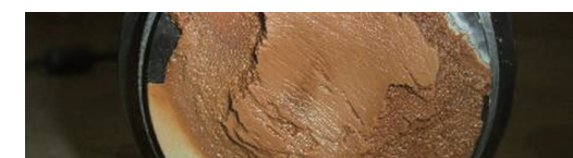
Debris Buildup Around the Detection Section
