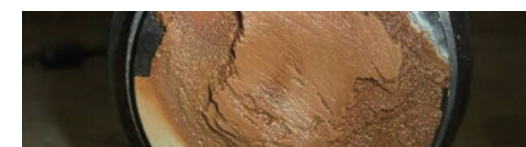
Debris Buildup Around the Detection Section
