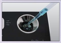
1. Fill the sample stage up to the fill line (approx. 3mL).
